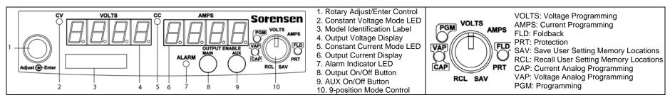
**XTR Front Panel Controls, Displays, and Indicators**
